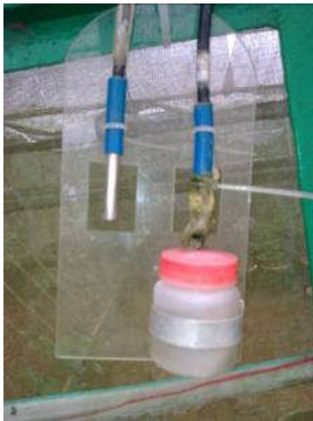
Pic 08. Wet & Dry Bulb thermometer sensors
