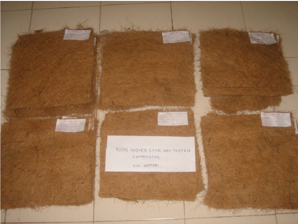
Fig: 7 Heavy Weight Non-Woven Coir Geo-Textiles Composite (950 g/m 2 )
