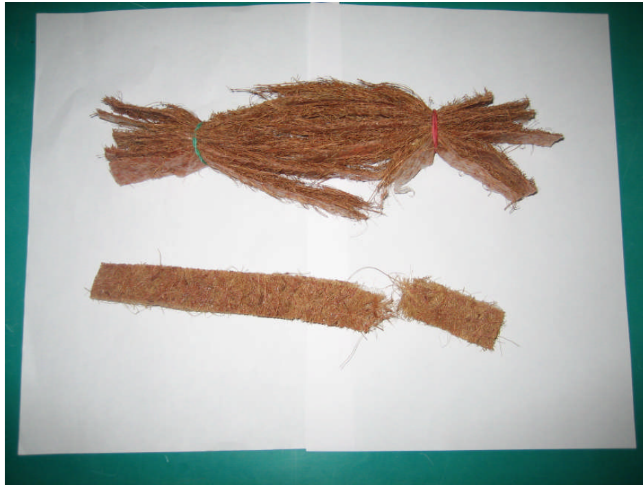
Fig: 3 Photograph showing the coir geo-textile composite specimen after tensile testing
