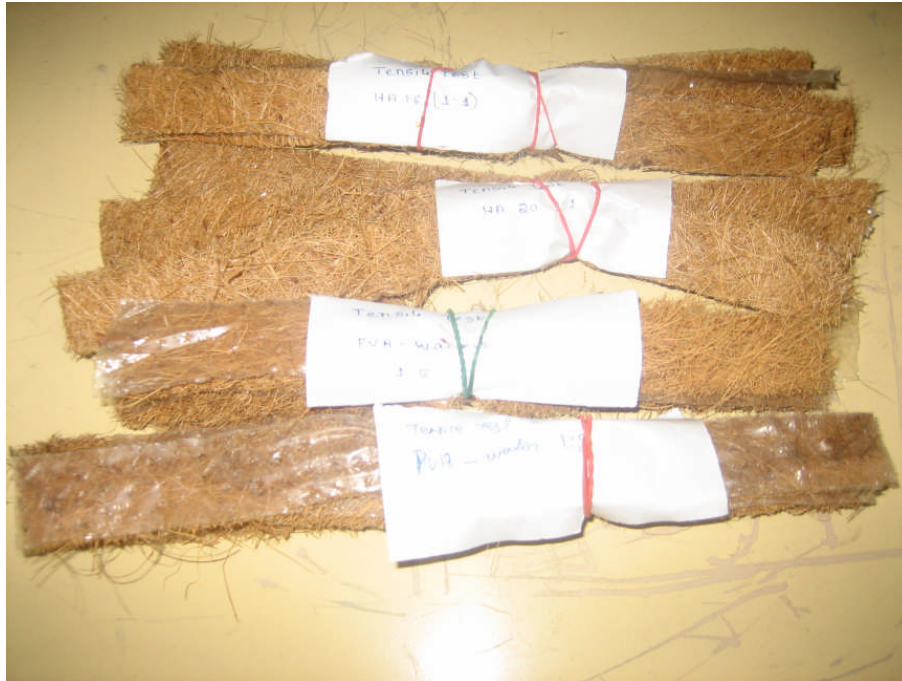
Fig: 7 Photograph showing coir geo-textile composite specimen with (PVA, HA 16, HA 20 and HA 24) after tensile testing
