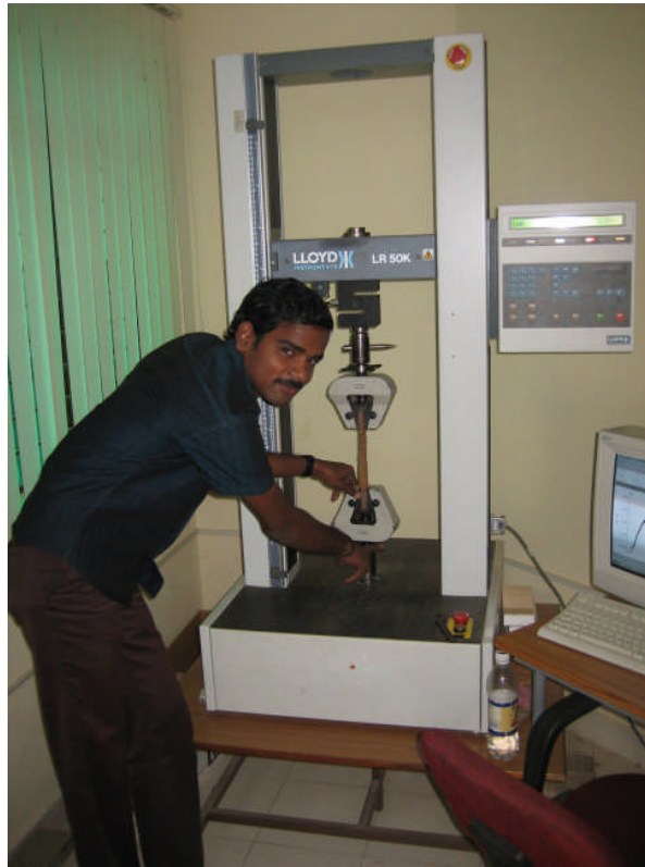
Fig: 1 Tensile Strength Test of Non-Woven Coir Geo-Textile Composites Specimen
