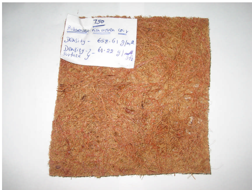
Fig: 3 Photograph showing the coir geo-textile composite specimen after tensile testing
